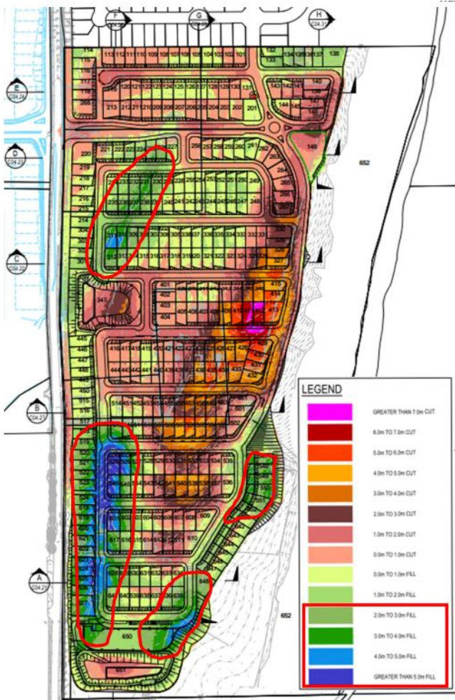
Figure 13: Proposed bulk earthworks identifying fill that would exceed 2m (outlined in red).
